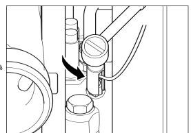
Extract the speed sensor and place on a clean surface to avoid collection of unwanted ferrous particles.
