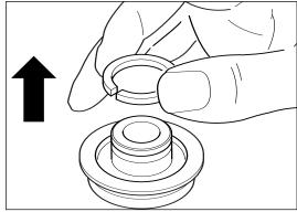
Remove and discard the oil baffle (33) \*.
