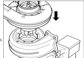
Turbine housings and CHRA assemblies are heavy. Always use safe lifting methods.
