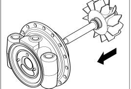
Support the assembly turbine wheel (6) in a suitable fixture.
