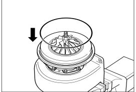
Inspect internal profile of compressor housing for scoring damage due to possible contact with compressor wheel. Move to *Cleaning of Housings* if deposits remain.
