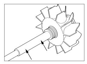
Inspect for cracked, bent or damaged blades.
