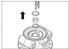
Turn the bearing housing over and repeat the process of bearing removal at turbine end.
