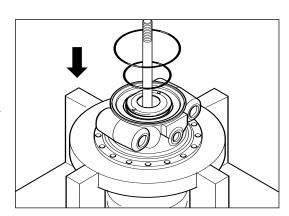
Fit the new split ring seal, compressor (16)  $\star$  to new oil slinger (31)  $\star$ .
