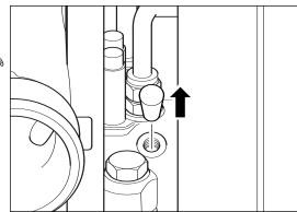
Prior to inserting speed sensor ensure it is clean and unable to collect magnetic particles as it is inserted. The sensor is designed to seal directly in the bearing housing without any supplementary sealing. Do not fit an o ring or washer.
