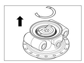
Remove the thrust bearing (12) \* and discard.
