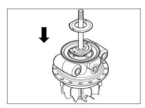
Lubricate and install new o-ring seal, compressor (32) \*. Install new o-ring seal (27) \* to liquid cooled bearing housings at this stage.
