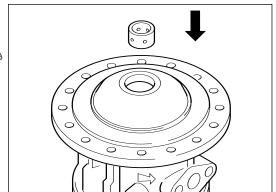
Fit outer retaining ring (64) \* with bevelled edge facing the bearing.
