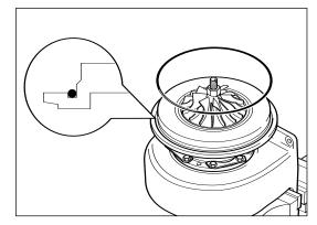
HX82 options with aluminium compressor housing may have an o-ring fitted. Where fitted, the o-ring groove will be machined in the compressor housing.
