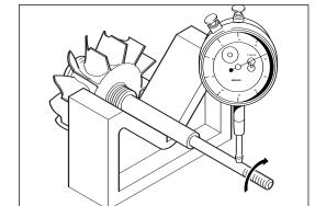
Inspect split ring seal, turbine (13)\* groove walls for wear. If groove width exceeds recommended maximum of 1.70 mm (0.067 in) replace assembly.
