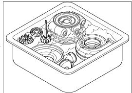
Dry the components using compressed air.
