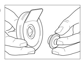
Using a small screwdriver, release oil baffle (33)\* from its light fit location in the oil seal plate (43) and discard.
