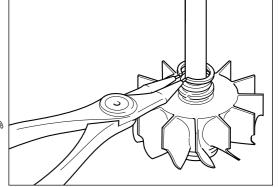
Where fitted, use circlip pliers Part No. 56663 to remove heat shield retaining ring (95)
