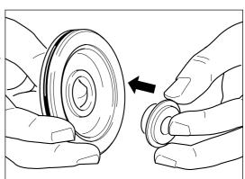
Press fit oil baffle (33)\* into oil seal plate (43).
