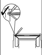
Place the turbine and bearing housing assembly on a clean surface. To refit compressor housing, loosely fit Vband clamp. Carefully locate the compressor housing over the compressor wheel.
