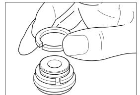
Remove the thrust bearing (12)\* from its pin locations and discard.
