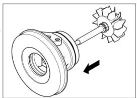
Support the assembly turbine wheel (6) in a suitable fixture.
