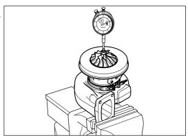
Check compressor end radial movement using a dial gauge. Ensure clearance lies within MIN/MAX TIR (Total Indicator Reading) values shown on **Service Data Sheet**.
