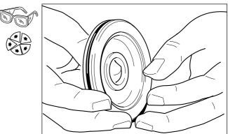
Fit new split ring seal/seals, compressor (16)\* to oil slinger (31).
