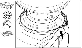
Check thrust clearance using a dial gauge. Ensure clearance is within MIN/MAX values shown on **Service Data Sheet**.
