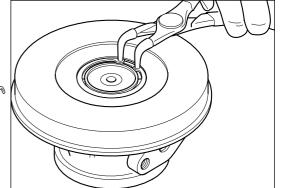
Remove oil seal plate assembly using mole grips.
