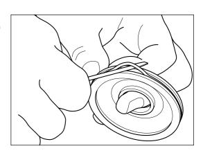
Remove and discard split ring seal / seals, compressor (16)\* from oil slinger.
