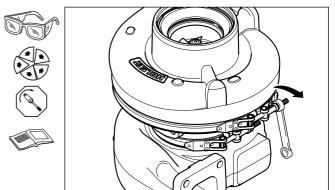
Ensure rotor assembly freely rotates.
