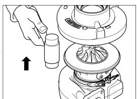
Inspect internal profile of compressor housing for scoring damage due to possible contact with compressor wheel. Move to *Cleaning of Housings* if deposits remain.
