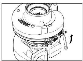
Ensure rotor assembly freely rotates.
