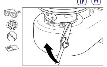
Ensure rotor assembly freely rotates.
