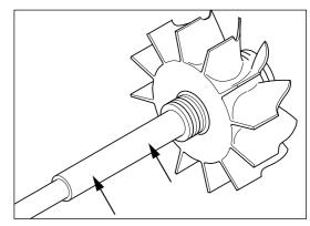
Inspect for cracked, bent or damaged blades.
