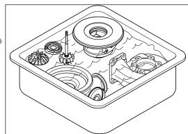
Dry the components using compressed air.
