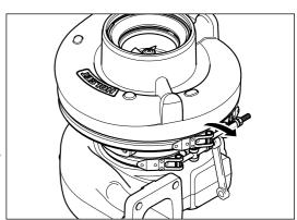
Using a soft hammer, tap turbine housing down against soft bench surface. As bearing housing and compressor housing assembly comes loose gently lift it out of turbine housing engagement
