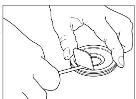
Remove and discard the o-ring seal, bearing housing (32)\*.
