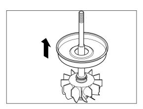
Carefully remove the split ring seal / seals, turbine (13) \* and discard.
