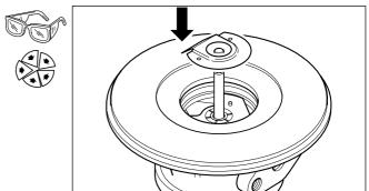
Apply a small amount of engine oil to the o-ring and insert the o-ring seal, bearing housing (32) \*.
