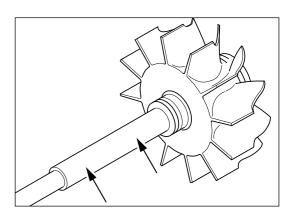
Inspect for cracked, bent or damaged blades.
