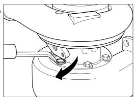
Ensure rotor assembly freely rotates.
