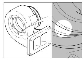
To replace turbine housing position V-band clamp (where fitted) over the bearing housing and align indelible ink marks applied during disassembly.
