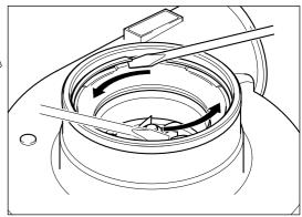
Following cleaning of the compressor housing, locate a new type of inlet baffle onto the location ledge of the compressor housing inlet.
