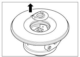
Remove the thrust bearing (12) \* from its pin locations and discard.
