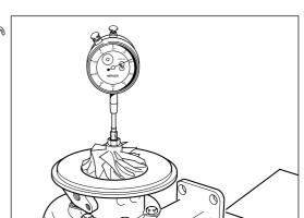
Check compressor end radial movement using a dial gauge. Ensure clearance lies within MIN/MAX TIR (Total Indicator Reading) values shown on **Service Data Sheet**.
