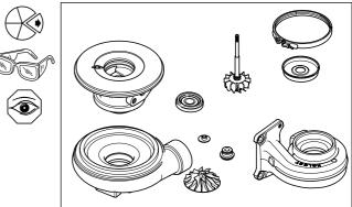
Soak the components in a non-corrosive low flash point metal cleaner to loosen deposits.
