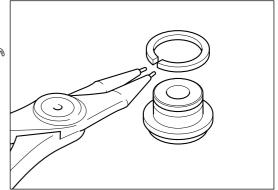
Install oil slinger (31) into oil seal plate (43).
