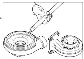
Scale like deposits, if any, must be removed by using a non metallic bristle brush. After removing the deposits, re-wash and dry the components.
