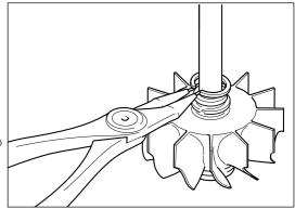
With bearing housing (4) on a flat clean surface, use circlip pliers Part No 56662 to remove insert, retaining ring (66).
