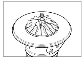
Inspect internal profile of compressor housing for scoring damage due to possible contact with compressor wheel. Move to *Cleaning of Housings* if deposits remain.
