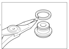
Remove and discard the o-ring seal, bearing housing (32) \*.
