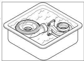
Dry the components using compressed air.
