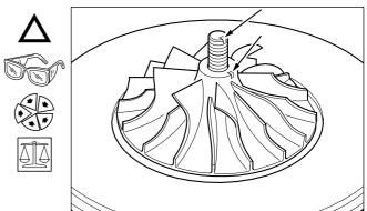
Brush the thread and nut face with an anti-seize compound to avoid loss of alignment during torque tightening.
