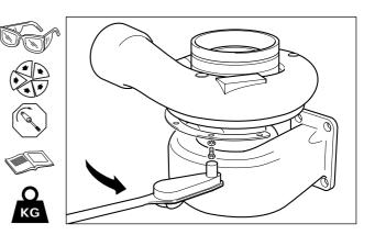
Ensure rotor assembly freely rotates.
