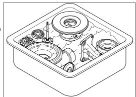
Dry the components using compressed air.
