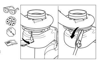
Ensure rotor assembly freely rotates.
