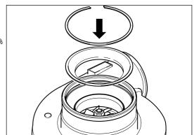
Hold one end of the retaining ring in position in its compressor cover groove. Press the remainder of the retaining ring into position using free hand.
