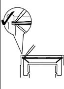
Place the turbine and bearing housing assembly on a clean surface. To refit compressor housing, lubricate new o-ring seal (41) with clean engine oil and install into retaining groove. Loosely fit V-band clamp (where fitted). Carefully locate the compressor housing over the compressor wheel.
