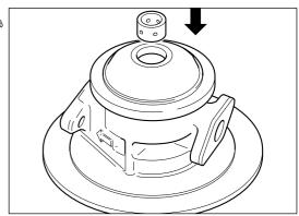
Fit the outer retaining ring (64) \* with the bevelled edge facing the bearing.
