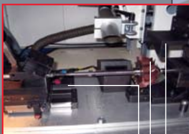
Laser to verify thread presence
