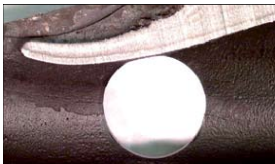
Fig 7 - Thermal crack looking from volute
