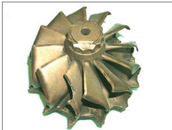
Fig 1 - Blade failure due to high cycle fatigue
