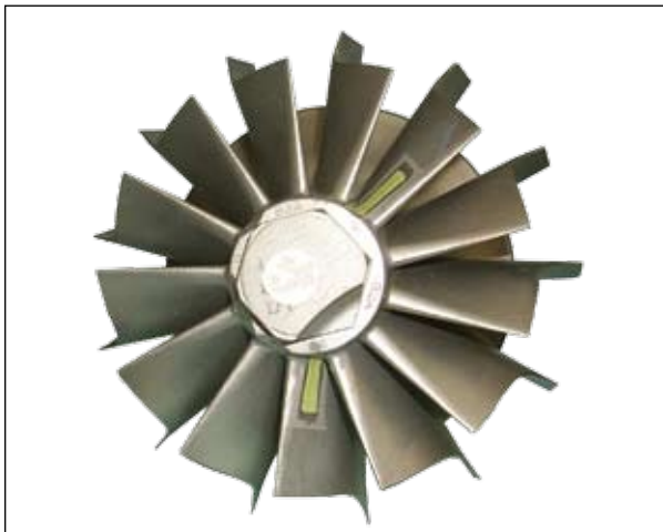
Fig 3 - Strain gauges on the identified most responsive blade and another blade. Tip-to-tip frequency response is the displacement of one tip due to a unit force at the same or another tip
