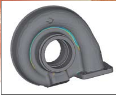
Fig 5 - Fatigue life plot (blue is lowest life)
