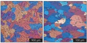
Fig 5 - Example of cast aluminium and wrought aluminium microstructure. Individual grains are observed as different colours. The magnification of the wrought alloy image is nearly ten times higher than that of the cast structure, demonstrating the finer grain detail of the wrought alloy.
