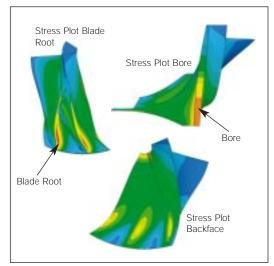
Fig 3 - Contour plot of stresses generated due to centrifugal loading, showing peak stresses in blade root and bore.
