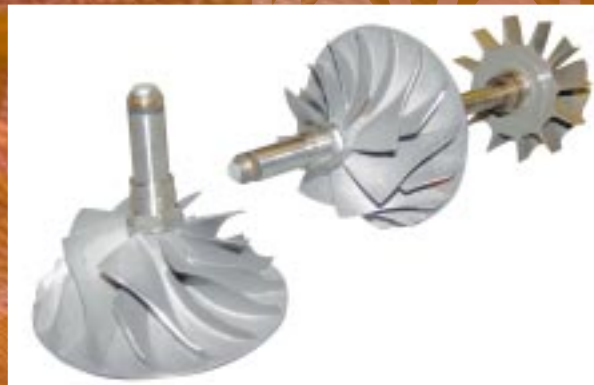
The instrumented rotor assembly with a strain gauged turbine and a transmitter mounted compressor.
