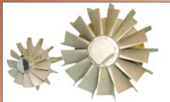
Turbine Wheels with strain gauge attached.
