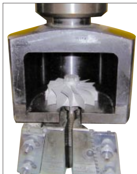
Tensile testing the friction weld joint.
