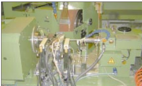
Finish grinding the shaft & wheel - showing steady rest and in process gauges used to maintain shaft diameter tolerances.
