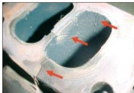
Fig 2 - Cracking of a turbine housing
