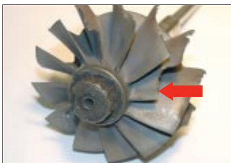
Fig 1 - Fracture of a turbine wheel
