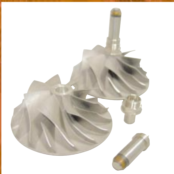
The modified compressor wheel houses the precision nut and radio transmitter for non-contact, data transfer.
