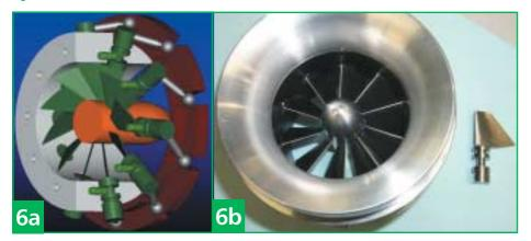
For any set vane angle, the compressor map looks very narrow. This is simply due to the presence of the vanes, which is why Holset uses a vaneless diffuser for standard non VGCs. It was found in testing that the incidence angle on to the leading edge of the vanes can result in a major loss of efficiency when operating away from the design point.
