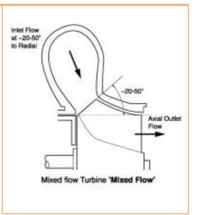
itself need to be of 'mixed flow' configuration, or canted over in a way that could hinder installation in a vehicle's congested engine compartment. Holset's collaborative work with Imperial College, London, on mixed-flow turbine technology has now finished. But there remains a good deal of investigative work still to do.
