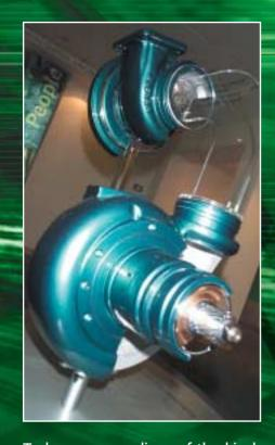
Turbocompounding, of the kind adopted by Swedish heavy truck manufacturers in recent years, is a technique involving use of a second power turbine. Located in the exhaust system, usually downstream of the turbocharger, it feeds additional power from the exhaust gas into the engine crankshaft mechanically, via a reduction gear train. It is also possible to harness the turbocompound's power output in some other form, for example to drive an electrical generator or an air compressor.
