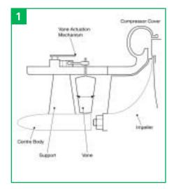
Figures 1 and 2 show diagrams of axial inlet guide vanes and radial inlet guide vanes respectively.
