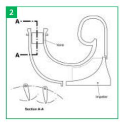
Varying the inlet flow angle to the compressor usually involves a row of small vanes whose angle can be controlled. The vanes can be positioned axially upstream of the compressor inlet, or radially upstream ahead of a radial-toaxial inlet - that switches the flow from a radial to an axial direction – ahead of the compressor inducer.
