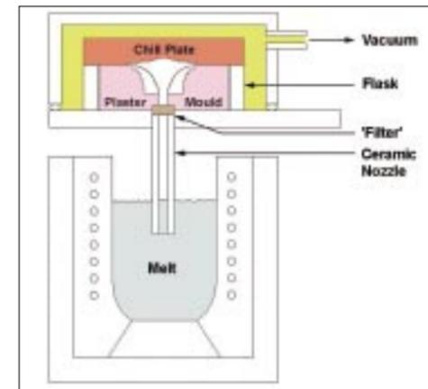
Fig 4 - Schematic of atmospheric pressure furnace configured for plaster mould casting process.
