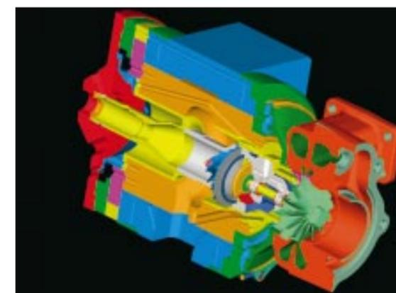
Fig 3 - Mid-range dynamometer section view
