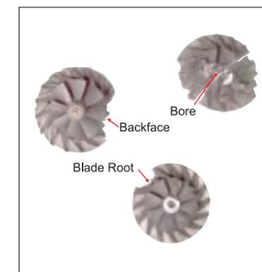
Fig 2 - Three typical impeller failure modes
