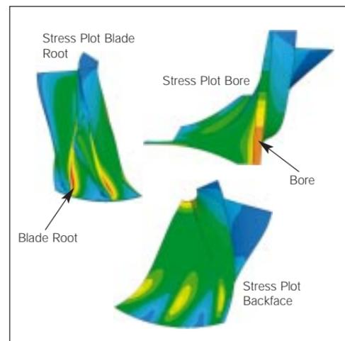
Fig 3 - Contour plot of stresses generated due to centrifugal loading, showing peak stresses in blade root and bore.
