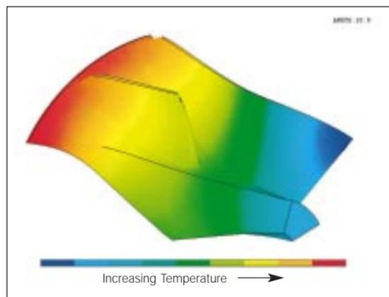
Fig 2 - Temperature distribution in a radial impeller.
