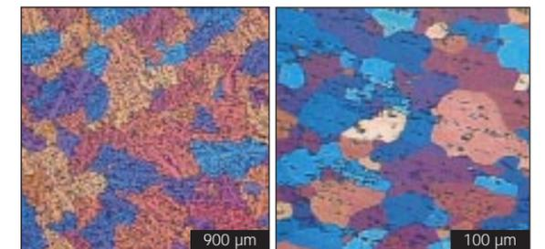
Fig 5 - Example of cast aluminium and wrought aluminium microstructure. Individual grains are observed as different colours. The magnification of the wrought alloy image is nearly ten times higher than that of the cast structure, demonstrating the finer grain detail of the wrought alloy.
