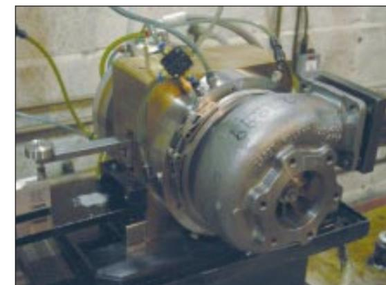
Fig 2 - Mid-range dynamometer with turbine housing fitted.
