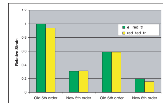
Fig 6 - Predicted and measured relative blade strain from old and new housing
