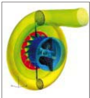
Fig 6 – Example of the CFD mesh used
