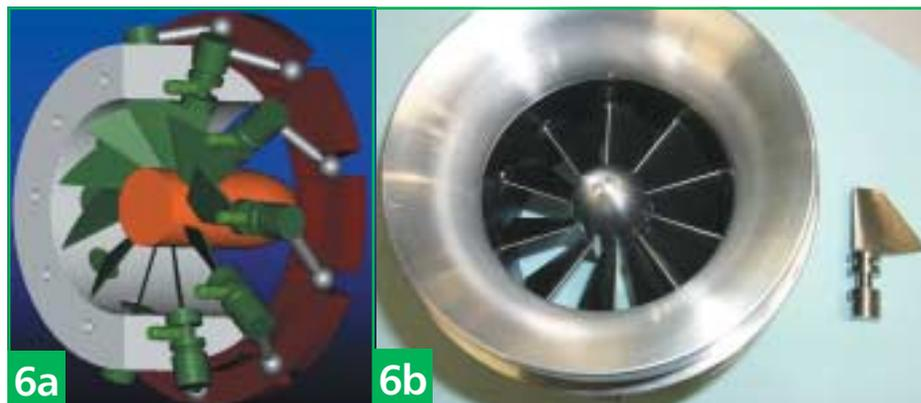
Holset's experiments with variable-vaned diffusers showed that overall map width can be varied significantly, mainly by modifying the 'choke' flow of the compressor map. 'Overall range' defines the difference between the surge flow with the vanes in their most closed position and choke flow when the vanes are fully open.
