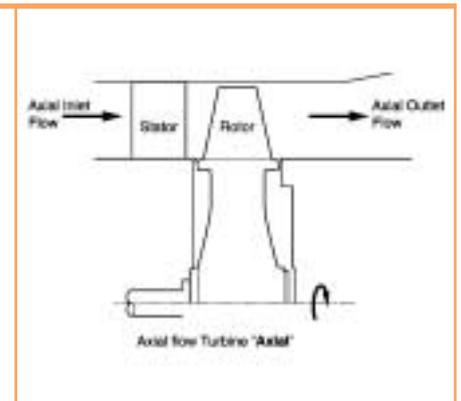
wheel. Consequently, smaller axial turbine wheels are usually of 'blisk' construction that is an integrated, one-piece, blade, disk and hub arrangement. However, it requires complex tooling and limits the designer in his choice of blade shapes more so than with a radial.
