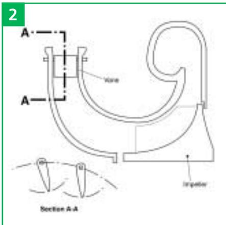
Varying the inlet flow angle to the compressor usually involves a row of small vanes whose angle can be controlled. The vanes can be positioned axially upstream of the compressor inlet, or radially upstream ahead of a radial-to-axial inlet - that switches the flow from a radial to an axial direction – ahead of the compressor inducer.
