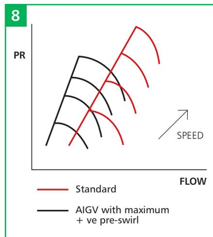
For any set vane angle, the compressor map looks very narrow. This is simply due to the presence of the vanes, which is why Holset uses a vaneless diffuser for standard non VGCs. It was found in testing that the incidence angle on to the leading edge of the vanes can result in a major loss of efficiency when operating away from the design point.
