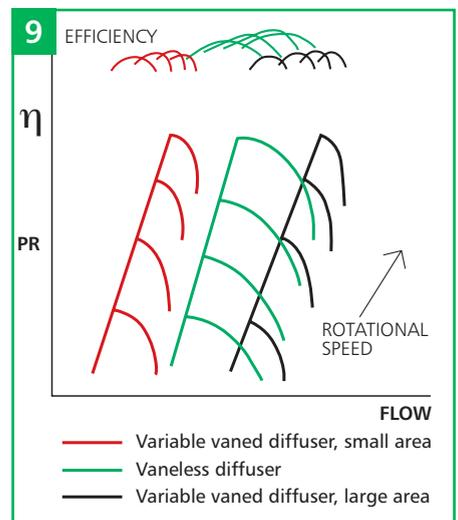
Although a moving sidewall vaneless diffuser has yet to be subjected to specific testing by Holset, regular experiments with diffuser width optimisation provide a good understanding of its effects. The surge line movement is not as great as with a variable vane diffuser or inlet guide vanes and again there is a trade-off between efficiency and map width. Typically, a narrow diffuser width gives good map width with low efficiency, and vice versa.
