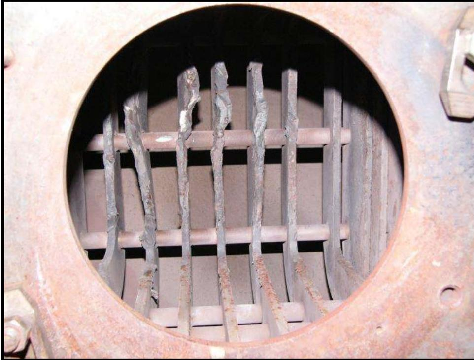
*This grating is made of thick steel bars and is known as the “bug catcher.” It is placed behind the turbine housing for Garrett® burst containment tests, to catch turbine wheels that may be ejected from their housings. This type of grating may be over-kill on a racing vehicle, but it illustrates the need for some type of structure to impede turbine wheels from escaping through the housing outlet.*
