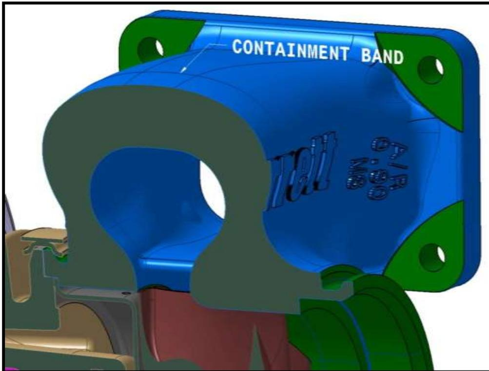
*The turbine housing containment band is visible in this cross-sectional view of a Garrett® GT55R. The containment band is the thickest section of the housing outside wall, radially outward from the wheel. If the wheel bursts, this thick wall needs to absorb the ballistic energy without failing in order to keep the wheel fragments contained within the housing.*
