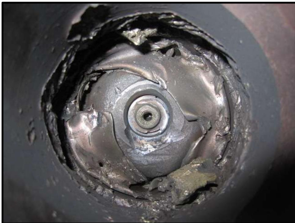
*This is the result of a successful turbine burst containment test. Note large chunks of wheel embedded in housing, and torn sheet metal heat shroud. Despite internal damage, exterior walls of the housing have remained intact.*
