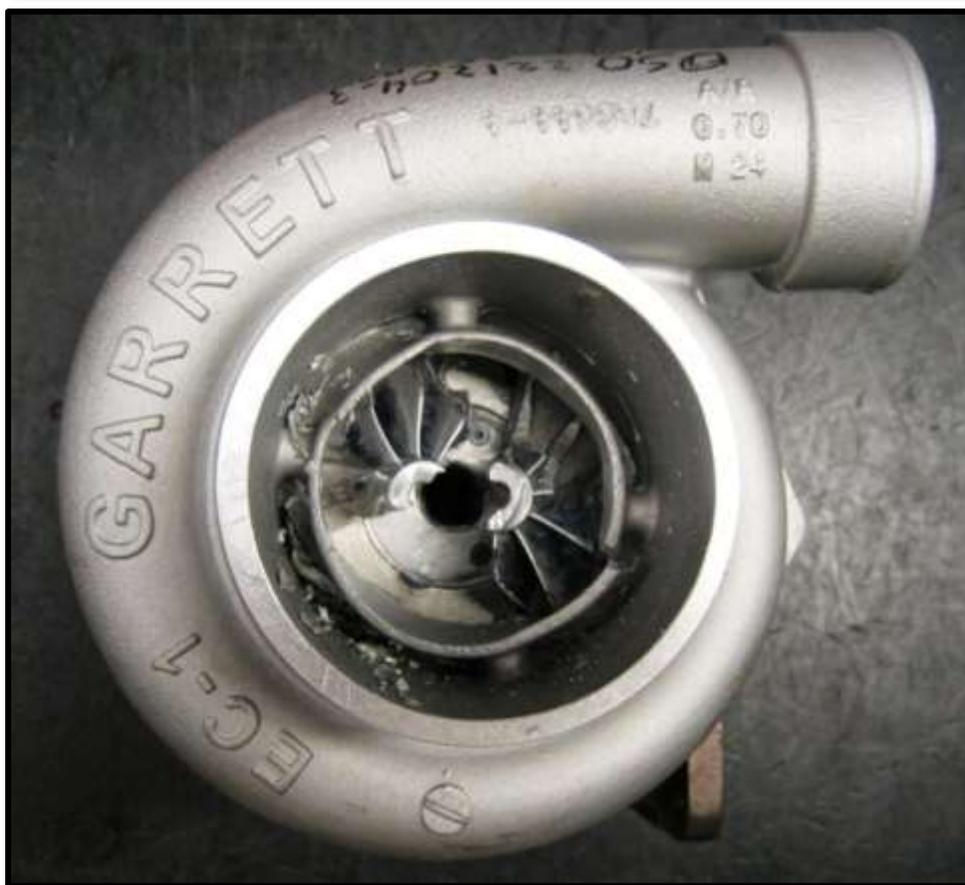
*The aftermath of a successful compressor burst containment test. Turbocharger is Garrett® GTX3582R. Hub burst was induced intentionally and wheel has fractured into two main pieces. Shroud contour wall between wheel and port has absorbed most of the burst energy through deformation. Outer housing wall and containment band remain unaffected.*
