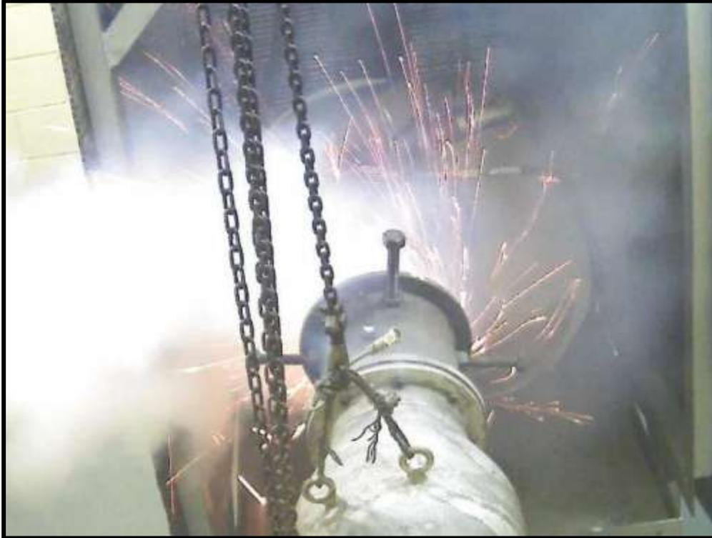
*Burst containment testing can get exciting! This still image was taken from video of a Garrett® GTX3076R compressor housing containment test. The turbocharger is barely visible behind the cloud of sparks; the object in the foreground is the turbine outlet pipe that collects the exhaust gases. After the compressor wheel burst, the turbine wheel contacted the turbine housing, causing the sparks.*
