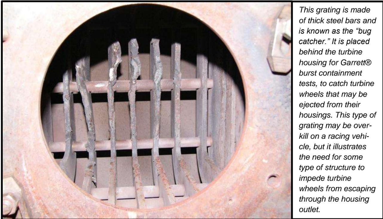
*This grating is made of thick steel bars and is known as the “bug catcher.” It is placed behind the turbine housing for Garrett® burst containment tests, to catch turbine wheels that may be ejected from their housings. This type of grating may be over-kill on a racing vehicle, but it illustrates the need for some type of structure to impede turbine wheels from escaping through the housing outlet.*
